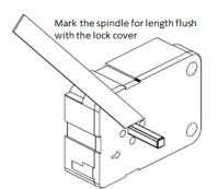
The length of the spindle can be precut to a length equal to Door Thickness (DT) + 1.75"
