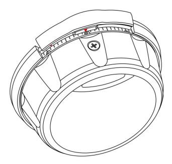
Step 3: Now rotate the SpinDial to the right until it comes to a stop (within one revolution)When the SpinDial comes to a stop the lock is open.
