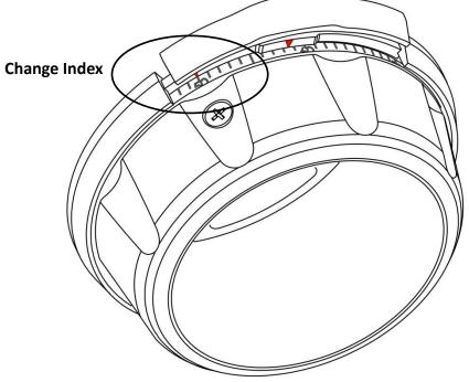
Step5: Rotate the SpinDial 4 times to the left, stop when you align the number "50" with the **Change Index.**
