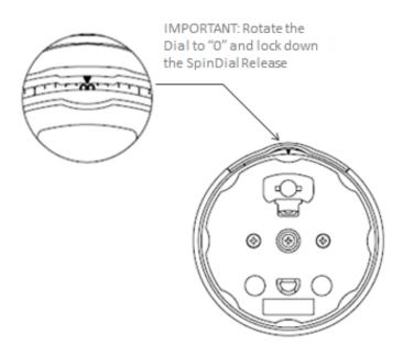
Step 2: Take note of the 3 ports (holes) surrounding the spindle insertion point on the lock cover as pictured below. These "Locator Ports" will be used to position the cam inside the lock correctly for SpinDial access.
