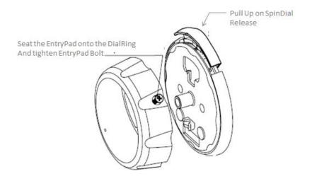
Step 5: Now rotate the SpinDial back to "00" and lock down the SpinDial release.
