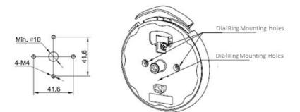
Note: In most safe installations, there are only two DialRing mounting holes, either aligned vertically or horizontally. Two bolts are adequate to secure the DialRing in place.
