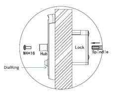
Step 15: IMPORTANT: Now from the Lock body side, tighten the small Phillips head screws to lock the spindle into place at the cam.
